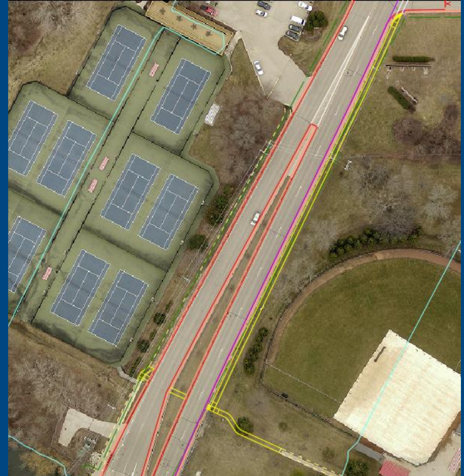
Proposed: Complete connection of sidewalk and add pedestrian crossing at WIS 32 to get access to west side and Smeds Tennis Center
